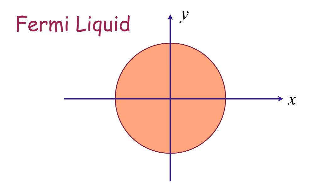
In momentum space, Fermi surface separates occupied and empty electron states
