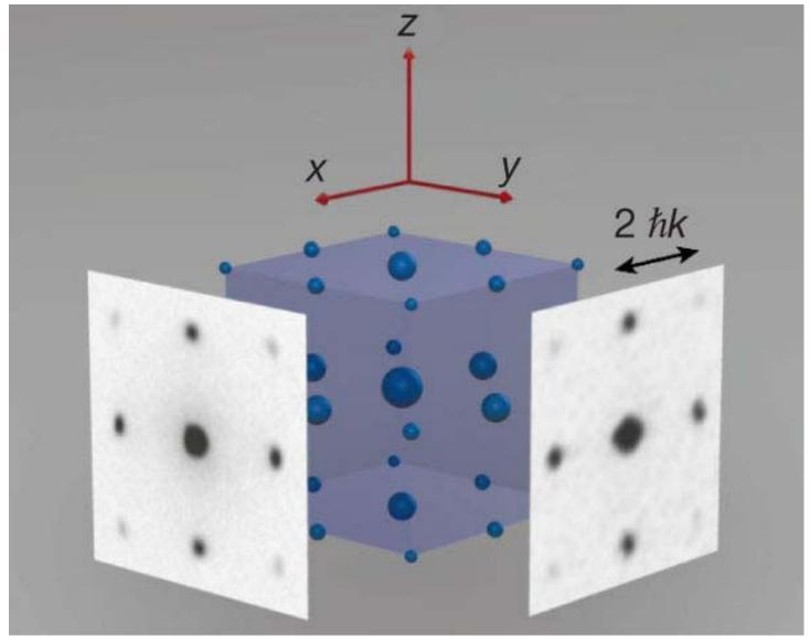
Schematic three-dimensional interference pattern with measured absorption images taken along two orthogonal directions. The absorption images were obtained after ballistic expansion from a lattice with a potential depth of  $V_0 = 10 E_r$  and a time of flight of 15 ms.
