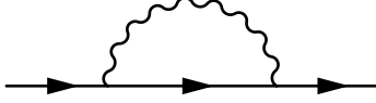
FIG. 6. Feynman diagram for the self-energy correction. The solid line with arrow represents F or G fermion propagator and the wiggly line represents electric field propagator. The interaction vertex is given by equation (3.12). This diagram is evaluated in equation (3.18).
